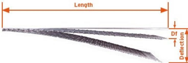
The top is a cantilevered straightedge and two scaled fabrics, one made with a 0.20" diameter wire, the other with a 0.10" diameter wire.
